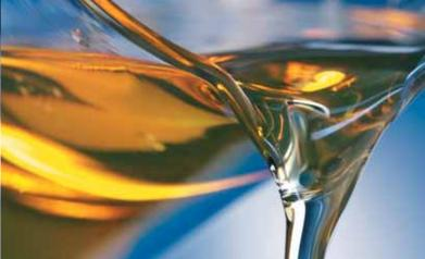
Hydraulic applications subject to very low temperatures or highly-fluctuating temperatures require oils with a high Viscosity Index to achieve good viscosity-temperature behaviour (little temperature-related changes to viscosity).
