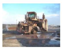
A slab carrier caught on fire. The equipment was using mineral oil hydraulic fluid.
