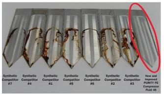
New and Improved PURITY FG Compressor Fluid shows much better varnish control than that observed for the competitive synthetic products.
