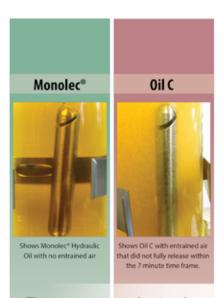
This test measures the time for entrained air content to fall to a relatively low valve.
