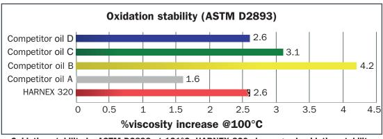
Oxidation stability by ASTM D2893 at 121°C. HARNEX 320 shows good oxidation stability under extended heating and oxidative conditions, promoting long service life.
