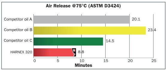
HARNEX 320 provides rapid air release, to maintain lubricating film integrity.
