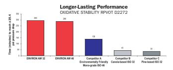
ENVIRON AW has greater resistance to oxidation and retains its fresh oil properties longer for fewer hydraulic fluid changes
