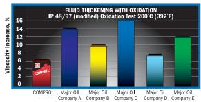
COMPRO's stronger oxidation resistance also reduces oil thickening, which can improve compressor efficiency and lower energy consumption costs.
